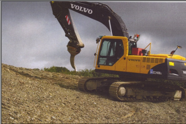
Inset 4 Tracked excavator with single rigid tine (Left) and Single rigid tine in use (Right)
